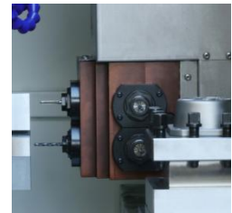
Live tooling on Y axis (optional)
